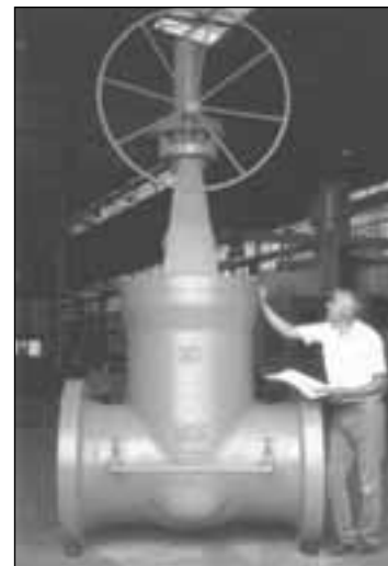
Pressure Seal Gate Valve. Class: 600#. Size: 30"
