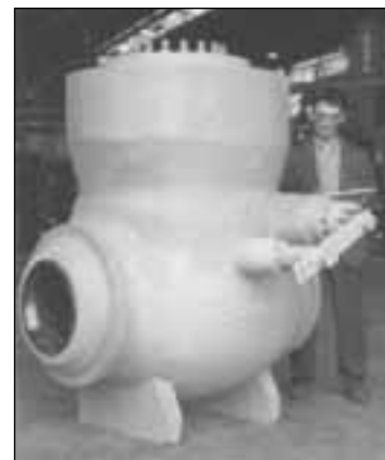
Pressure Seal Swing Check Valve. Class: 2500#. Size: 20"
