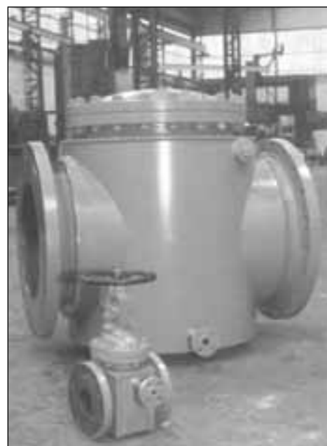
Jacketed Valves, Gate and swing check.
