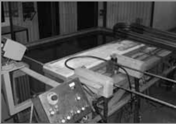
Electric resistance heat treatment with controlled temperature by an automatic Infra-Red-Camera
