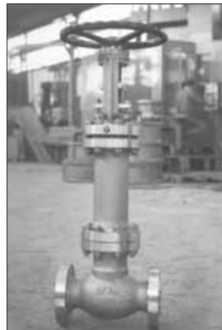
Bolted Bonnet Globe Valve with Bellow. Class: 600 #. Size: 3".
