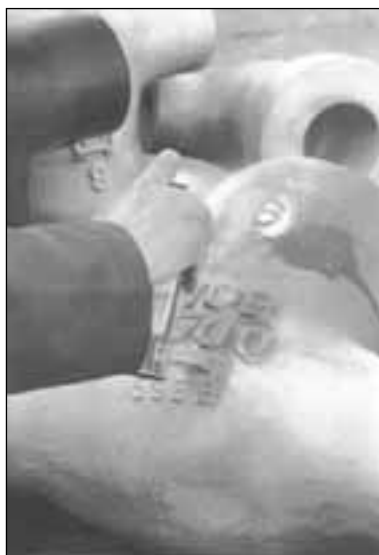
Dye penetrating inspection.
